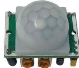
Fig. 2. Pir Sensor (Proximity Sensor): The Passive Infrared (PIR) sensor detects motion and presence. It is commonly used in security systems and automation.
