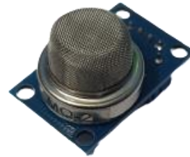
Fig. 3. MQ-2 Sensor (Gas Sensor): The MQ-2 sensor detects various gases and is used in applications like gas leakage detection.
