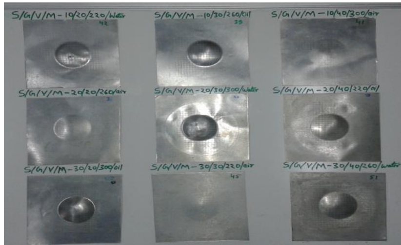
Figure 3: Tested samples in different conditions (S=SOD, G=Electrode GAP, V=Voltage, M=Medium)
