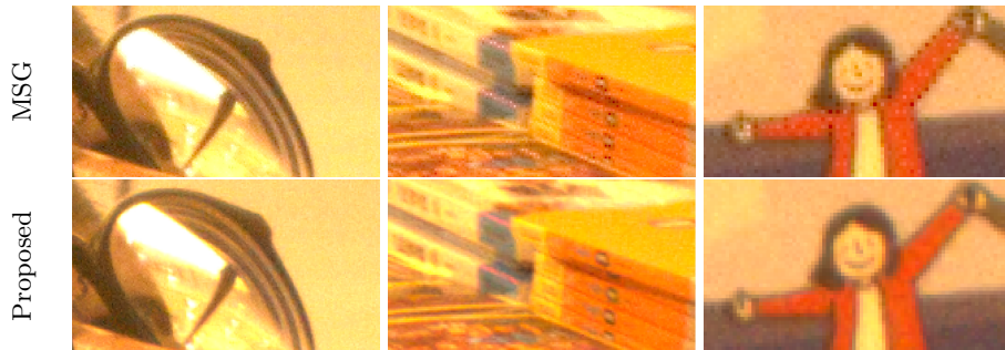
Fig. 6: Demosaicing on raw data captured from a smartphone
