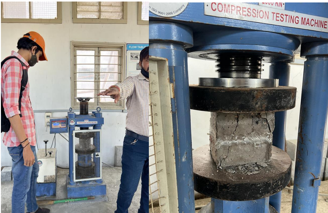
Fig:4 Testing of Cube
