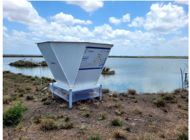
Figure 2. SODAR installed at the measurement point.
