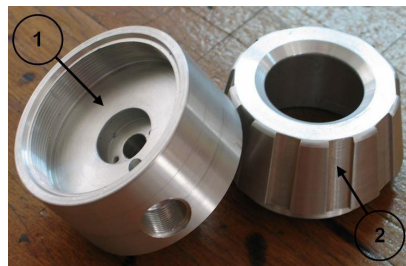
Fig. 8. Temperature transmitter enclosure (made of aluminium): 1- central part, 2- cover
