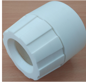
Fig. 9. Realized electronics enclosure using FDM procedure
