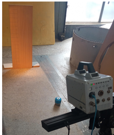
Fig. 25. Impact test using digital camera
